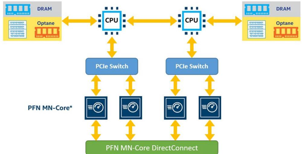
**Block diagram of PFN solution**
