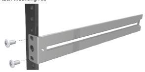
3. Mount the device in the rack, using the M6 screws provided in the Rack-Mounting Kit.
