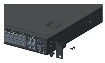
Mount the device in the rack, four additional M6 screws will be needed.
