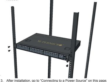
4. If installing multiple switches, mount them in the rack, one on top of the other.
