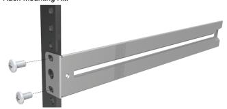
Mount the device in the rack, using the M6 screws provided in the Rack-Mounting Kit.
