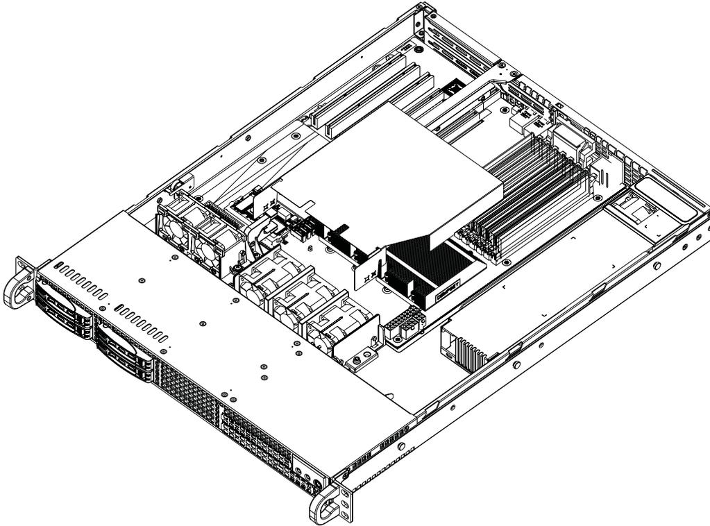
Figure 5-10: Air Shroud Installation
