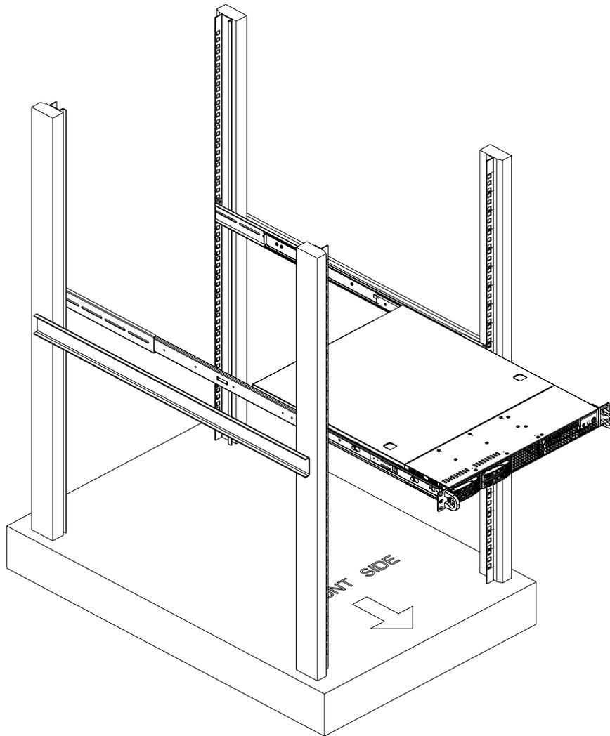
Figure 6-4: Installing the Chassis
