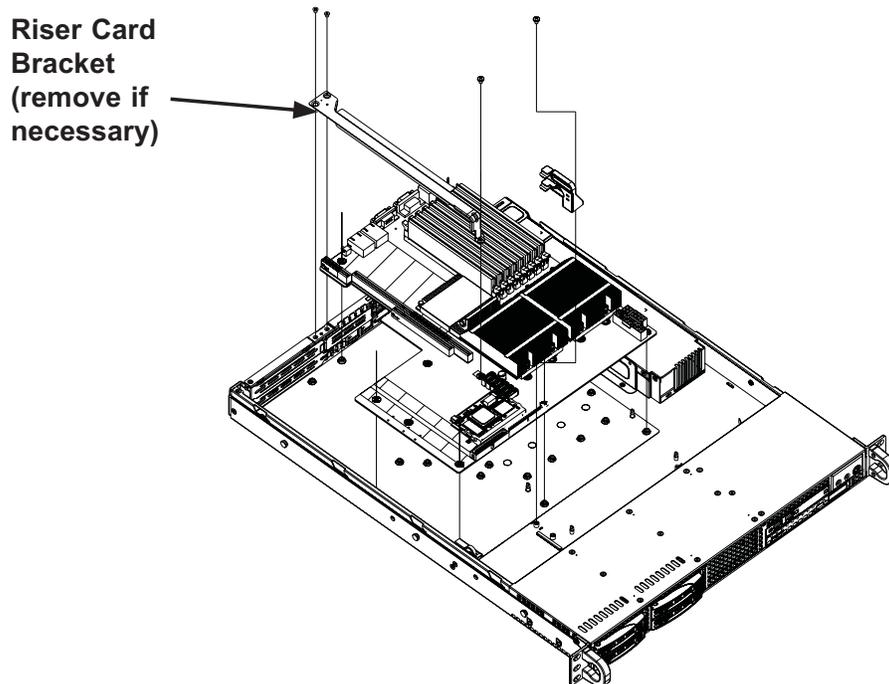
**Figure 5-7: Installing the Motherboard**
