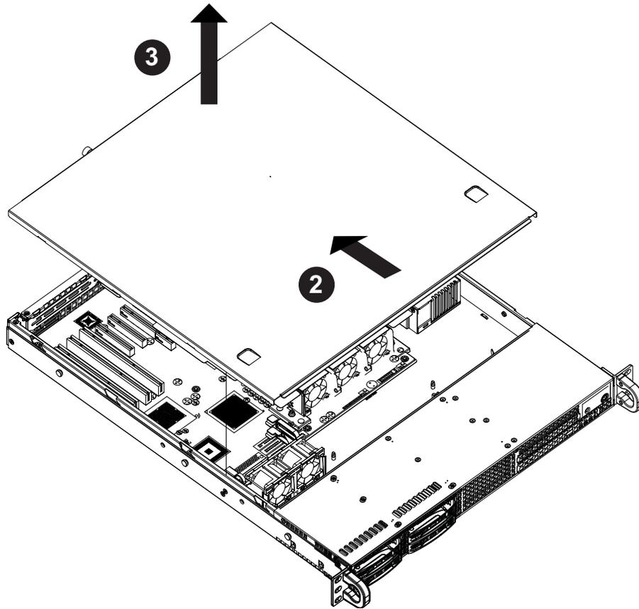
Figure 5-1: Removing the Chassis Cover
