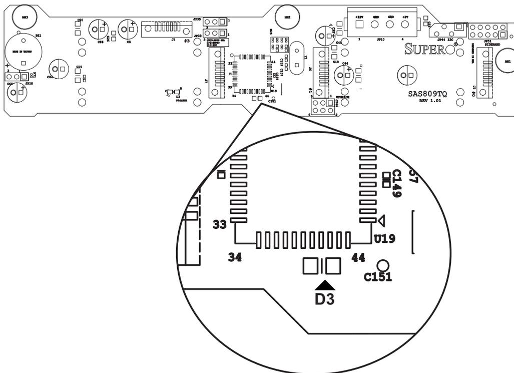
Figure C-3: Front LEDs
