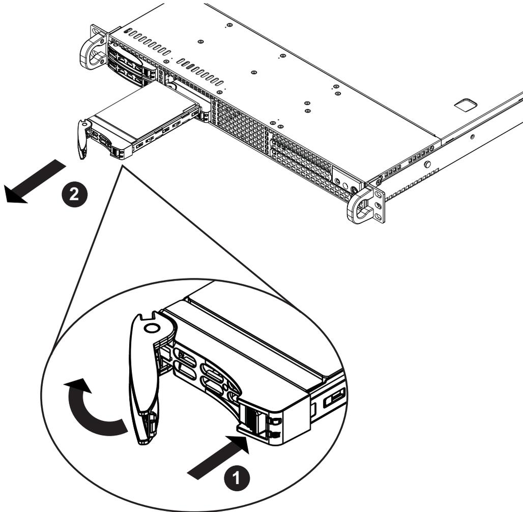
Figure 5-2: Removing Hard Drive
