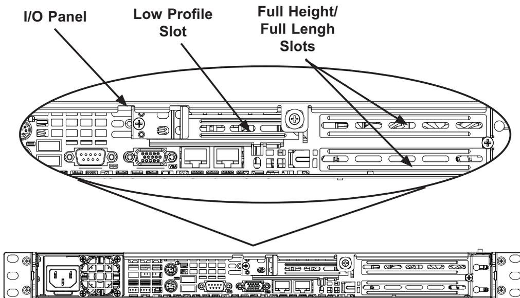
Figure 5-8: SC111 Rear - Full Height/Full Length Slots and Low Profile Slot
