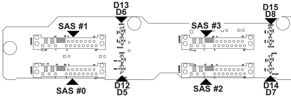
Figure C-4: Rear Connectors and LEDs
