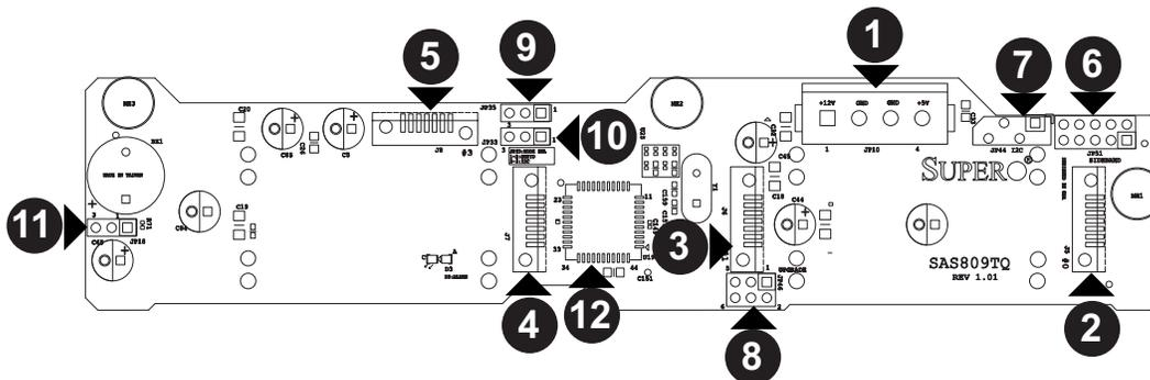
**Figure C-1: Front Jumpers and Connectors**
