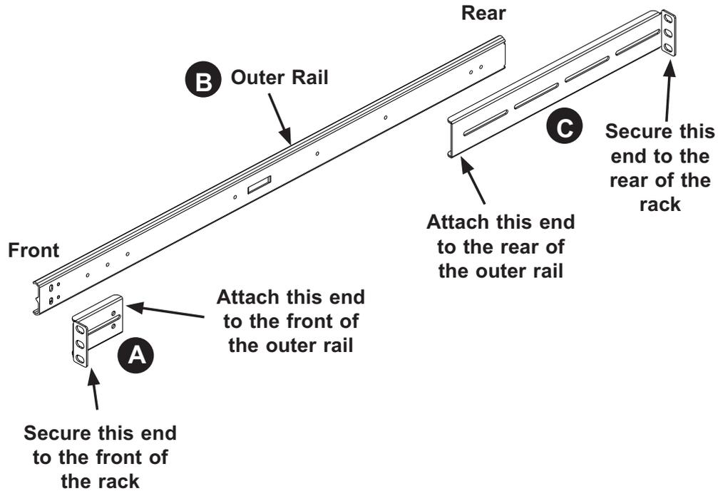
Figure 6-3: Assembling the Standard Outer Rails
