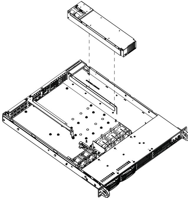
Figure 5-13: Removing the Power Supply
