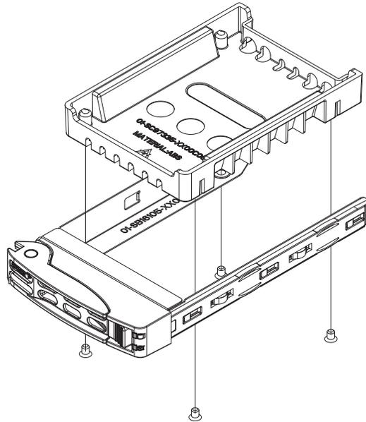
**Figure 5-3: Hard Drive Carrier**
