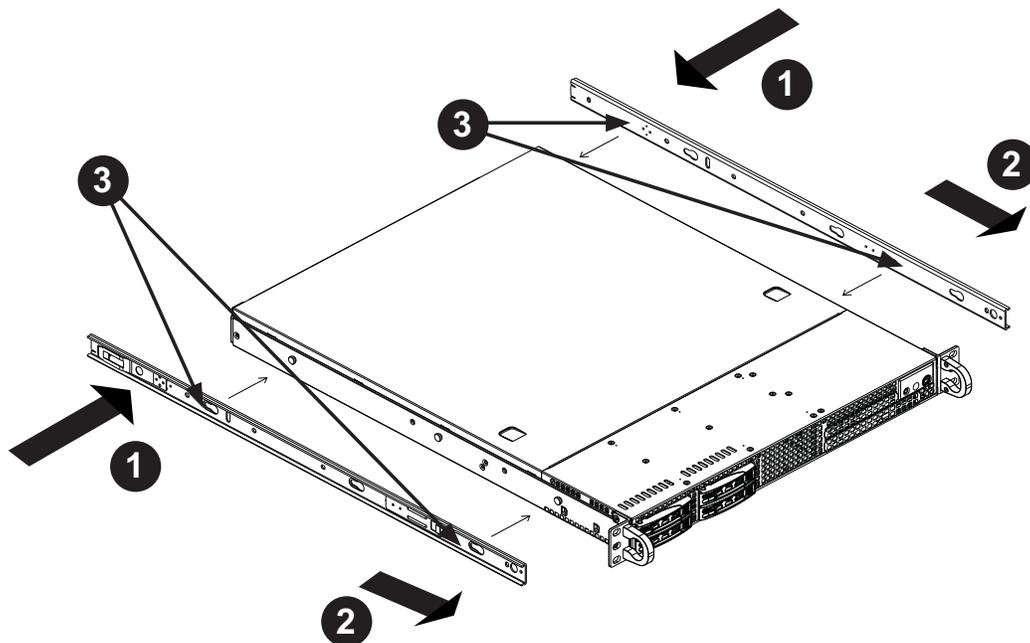
Figure 6-2: Installing the Inner Rails
