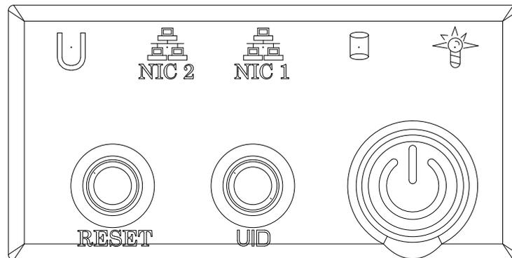
**Figure 4-1. Control Panel Buttons and LEDs**
