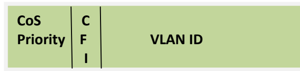
Figure QoS-4: VLAN Tag and CoS Priority
