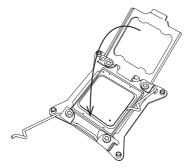
Push down and lock the lever labelled 'Close 1st'.
