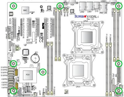
**Caution:** 1) To avoid damaging the motherboard and its components, please do not use a force greater than 8 lb/inch on each mounting screw during motherboard installation. 2) Some components are very close to the mounting holes. Please take precautionary measures to avoid damaging these components when installing the motherboard to the chassis.
