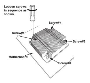
Note: For optimized airflow, please follow your chassis airflow direction to install the correct CPU heatsink direction. Graphic drawings included in this manual are for reference only. They might look different from the components installed in your system.
