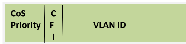
Figure QoS-4: VLAN Tag and CoS Priority
