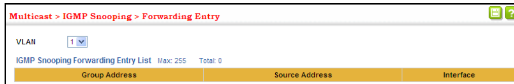
Figure 15-11: Showing Multicast Groups Learned by IGMP Snooping
