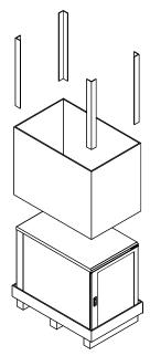
Remove the shipping container from around the rack unit by removing the corner supports and lifting the shipping container sides from around the rack unit.
