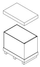
Remove the top of the shipping container to expose the rack unit.
