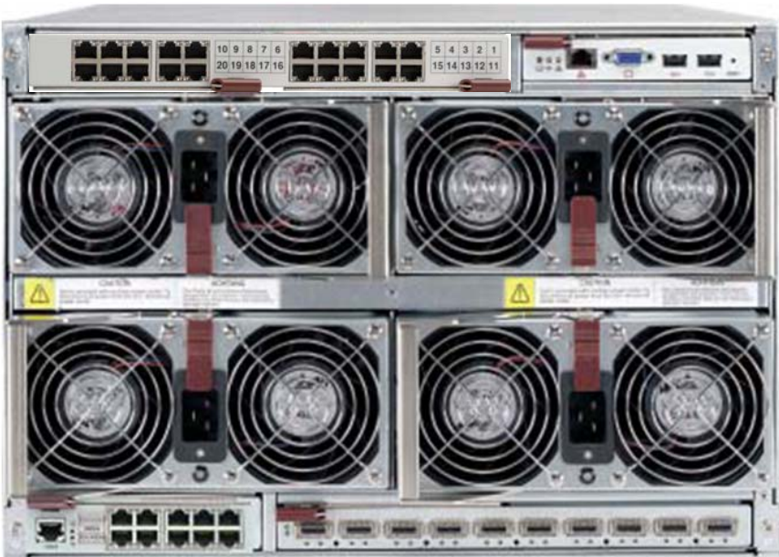
Figure 5-7. SBM-GEP-T20 Installed in Enclosure
