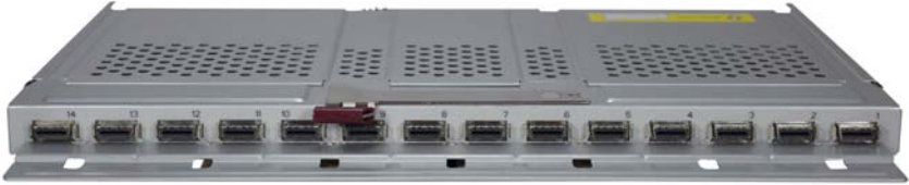
Figure 4-5. SBM-IBP-D14 InfiniBand Pass-Through Triple-Wide Module
