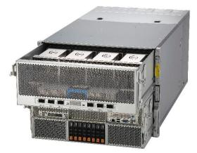
**1-socket system:** The leading system for the 1 socket systems for the SPEC Floating Point Speed result is the Supermicro SuperServer SYS-212HA-TN.
