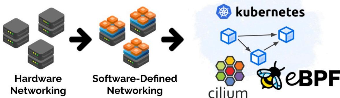
We recommend the use of Cilium as it provides a robust networking foundation for container networking. We also enable the ingress controller support in Cilium to facilitate applications that still require an ingress resource, instead of the more modern Gateway API.
