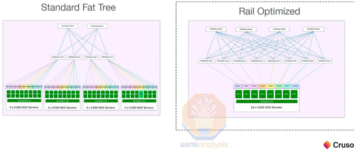
The advantage of a rail-optimized design is that each GPU can talk to a higher amount of distant GPUs through only 1 switch hop, compared to a fat-tree design. However, the rail-optimized design has a number of assumptions that aren't always in place:
