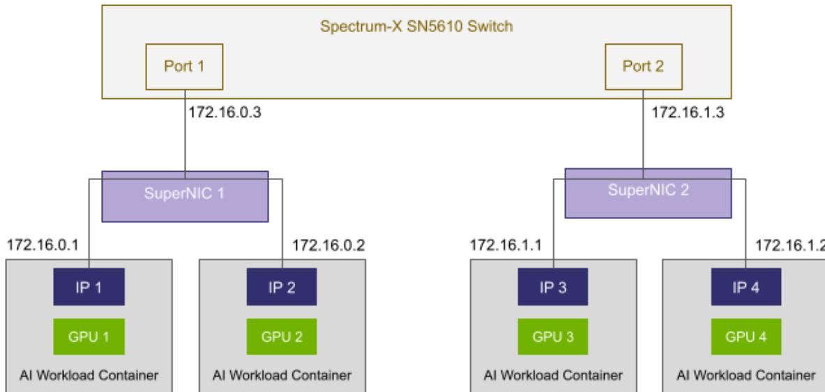
In both cases, the NVIDIA IPAM plugin is used to assign IP addresses to the additional network interface in a manner that is consistent with the Spectrum-X IP addressing scheme. When not using NVIDIA MIG to split the GPUs into even smaller instances, we recommend generating a Spectrum-X addressing scheme that uses /30 subnet prefixes per switchport. This gives you 4 usable addresses per link, one used by the switchport and 3 available to be used by VFs on the host.
