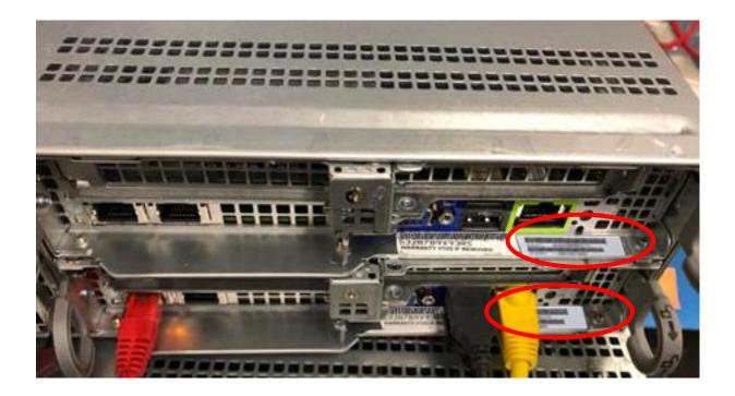
1U Twin system stickers will be above the first hard drive for each node. This is applicable when there is no service tag. Here is an example:
